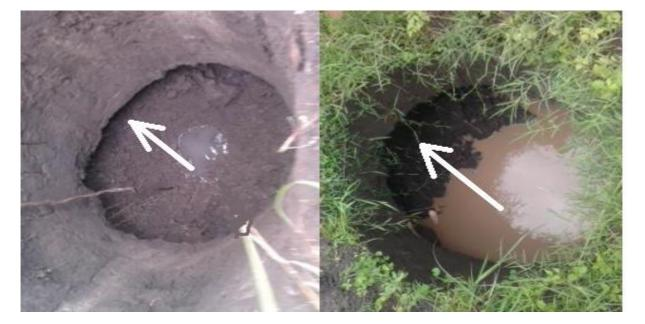
Figure 2: How pit collapse happens
