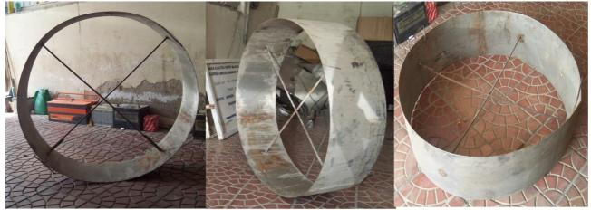
Figure 5: mold for pit lining
