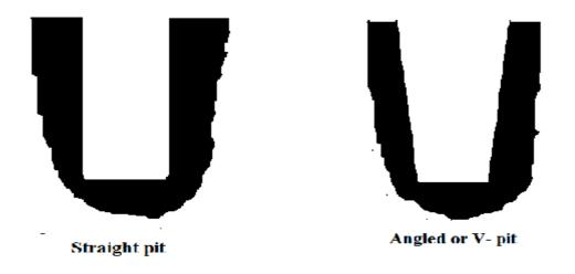
Figure 3: pit with different shapes
